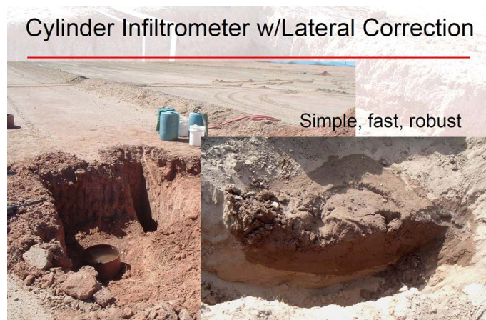
Figure 1. Measuring near-surface infiltration rate with a single ring infiltrometer and subsequent measure of lateral infiltration by visual inspection. (from Milczarek, M. 2022. State of the Art Techniques in Characterizing, Design and Operating Optimum Surface Spreading Groundwater Recharge Projects. 11th Int. Symp. on Managed Aquifer Recharge.)
