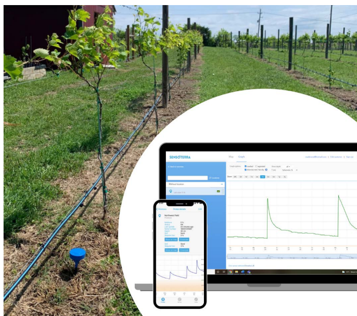
Sensoterra device in vineyard with the soil moisture data shown on a screen.
